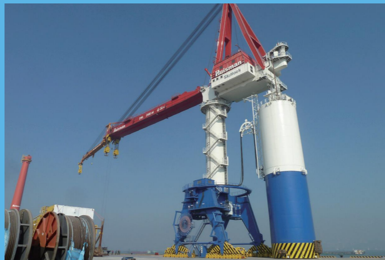
▲ 2400t Portal Slewing Crane (Awarded with Guinness World Records Certificate)
