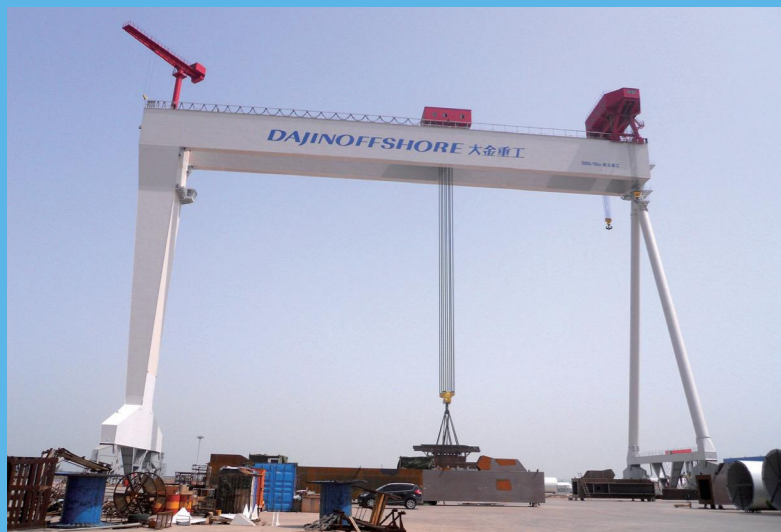
▲ Type Test of 1600t Shipbuilding Gantry Crane
